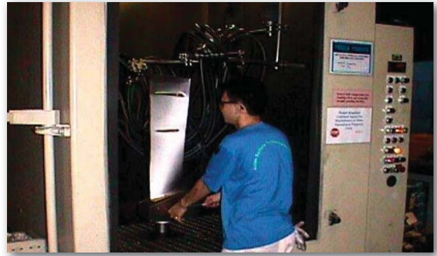
PEENING OF AIRFOIL TO RESTORE FATIGUE STRENGTH OF BLADE
